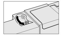
2. Insert the film cassette into the film chamber with the VEI (Visual Exposure Indicator) on top.
