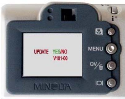
1. Insert the prepared SD memory card into the DiIMAGE F100, disconnect the AC adapter or remove the batteries and turn the main switch/mode dial to the playback mode position . Then connect the AC adapter or insert the batteries.
