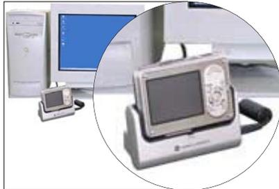
Copying via DiMAGE X1 (loaded on the Cradle CA-1) connected to PC
